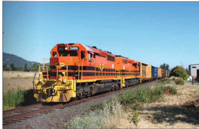
LEFT: Medford-Hornbrook Train 507 is running south through Talent, Ore., on June 20, 2016. CORP-rebuilt SD40-2s 3499 and 3498 are passing Chuck Roberts Park and will be tackling 3 percent grades ahead over Siskiyou Summit. The units are former CN SD40s.
