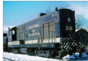
ABOVE: An F-M pocket of the Central of Georgia roster was just four H12-44s built in 1953. The option of m.u. connections suggests bigger things might have been planned. In Southern Railway's period of influence, CG 316 poses in Salem, Ind., on February 5, 1966. TOM SMART - LLOYD TRANSPORTATION LIBRARY
