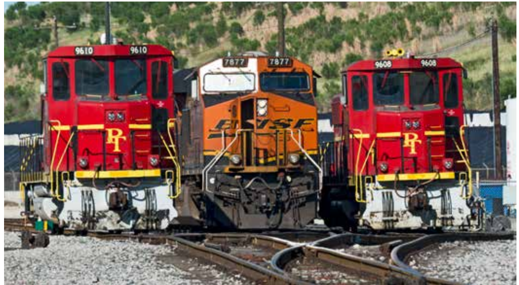
PTRA MK1500Ds Nos. 9610 and 9608 flank BNSF ES44AC at Pasadena Yard on the PTRA's South Shore Sub on April 8, 2017. The Morrison-Knudson units were the first to carry PTRA markings. Tom Kline
