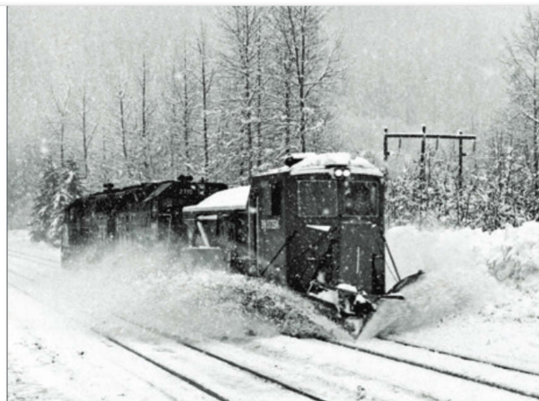
LEFT: Nothing is more spectacular than the Stevens Pass snow dozer making a "speed run" flinging snow in both directions from tracks. These unique snow-fighting machines are often confused with Jordan spreaders. BELOW LEFT: From the old Great Northern right-of-way along the flanks of Windy Mountain an eastbound Burlington Northern freight has the look of an N-scale model. The train is about to enter the eight-mile tunnel and this vantage point gives a clear view of how much elevation was eliminated by the new alignment. MARTIN BURWASH PHOTOS
