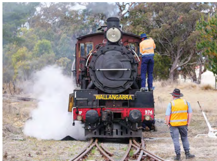
Left: The break-of-gauge yard at Wallangarra features a unique dual-gauge turning fork. On Saturday 12 August 2023, the crew of C17 974 takes the opportunity to blow down the boiler of 974 as it makes what would prove to be its last visit to the fork at Wallangarra. With the line now truncated to Stanthorpe (or perhaps Ballandean) the installation of a turning facility there will become a priority. Darren Tulk
