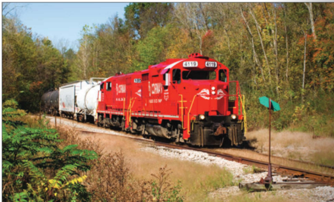
ABOVE: The unusual one-piece windshield of RJC 4119, a former Southern Pacific GP20E, is plainly seen in this view of a train leaving the east end of the W&LE Brewster yard. The signal protects the diamond crossing of the W&LE and RJCL.
