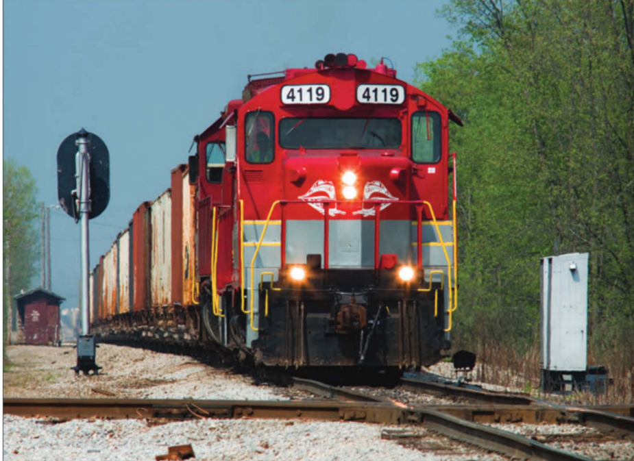
ABOVE: The unusual one-piece windshield of RJC 4119, a former Southern Pacific GP20E, is plainly seen in this view of a train leaving the east end of the W&LE Brewster yard. The signal protects the diamond crossing of the W&LE and RJCL.
