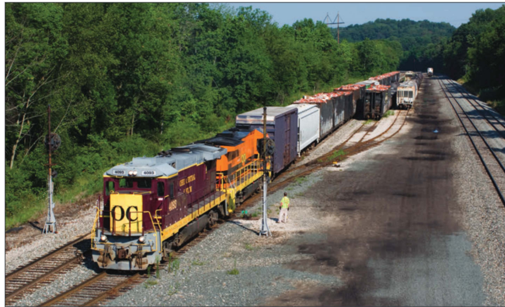
BELOW: As viewed from the Ohio State Highway 21 bridge, an Ohio Central crew is finishing an air test and is about to leave the CSX yard at Warwick. Both units started as Western Pacific U23Bs and were rebuilt by GE into Super-7s and sold to the Monongahela Railroad.
