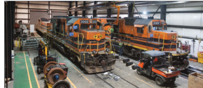
LEFT: The diesel doctors of Albany work on GP40P-2 no. 3002 (ex-Norfolk & Western 1382) and GP39-2 no. 2307 (ex-Santa Fe 3606) inside the railroad's two-bay shop on May 8, 2009.
