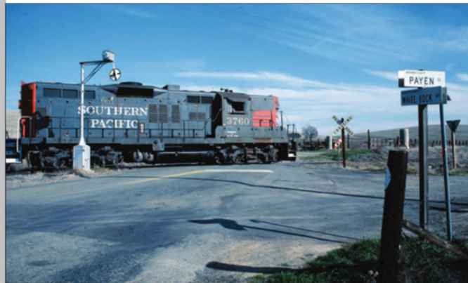
LEFT: In a classic scene that would soon disappear, SP GP9 No. 3760 leads the Placerville Turn past the wigwag crossing signal at White Rock on January 21, 1987. MARK ACUNA PHOTO BELOW LEFT: White Rock Road has become a busy thoroughfare, so reactivating the crossing required the classic wigwag for the crossing required the classic wigwag to be upgraded to modern flashing lights and gates in 2012. This part of the line features expansive views of the Sacramento Valley and Pacific Coast Range mountains 70 miles away.
