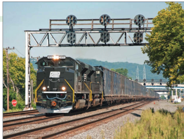
LEFT: Traditional Pennsylvania Railroad-style position light signals guide Norfolk Southern Train 64J on August 23, 2012, through Leetsdale, Pa. The unit trash train is bound for Oak Island, N.J. HARRY GAYDOSZ PHOTO
