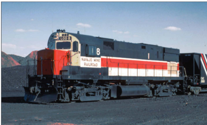
OPPOSITE: Non-powered "owl" No. LOD9 trails a northbound load towards the APS Four Corners Power Plant in Fruitland, N.M. The car was built as an Alco C425 for the Norfolk & Western, but had been ordered by the Wabash. JAMES HICKEY PHOTO
