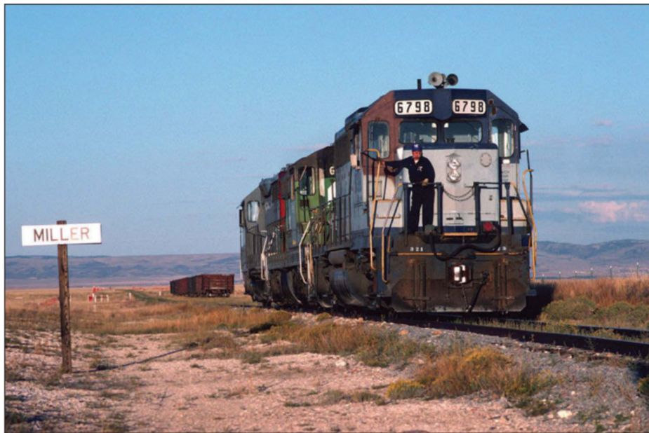
ABOVE: Brakeman Bob Johnson is protecting the reverse move as the trio of locomotives returns for the 16 loaded ore jennies that were left on the 2.5 percent grade at Windmill Hollow. The crew was forced to double the hill and leave the first eight loaded gondolas at Miller siding on September 9, 1996.
