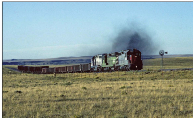
LEFT: The crew already has the trio of locomotives in Run 8 as it passes the namesake windmill at Windmill Hollow, just before tackling the 2.5 percent grade near Milepost 15 on September 9, 1996. On this day, the trio stalled on the grade, forcing the crew to double the hill and arrive into Laramie well after dark.
