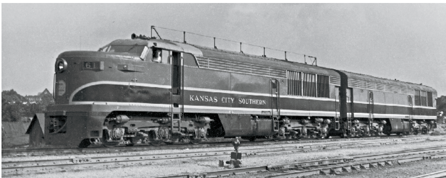
Kansas City Southern was one of seven buyers of 2,000 hp Fairbanks-Morse "Erie-built" units. The units derived their name from their assembly at General Electric's facility in Erie, Pa., when FM didn't have capacity at its Beloit, Wis., plant. A three-year-old cab-booster set rests at Shreveport, La., in July 1949. Harold K. Vollrath
