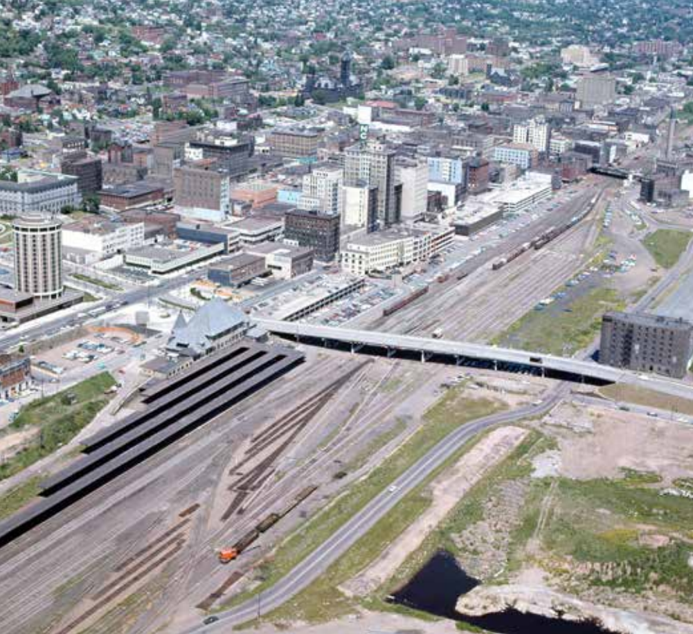
This aerial view of downtown Duluth circa 1971 shows work being done to reconfigure BN's Bridge Yard to better handle long trains of interchange from the DW&P. C&NW's nearly empty 5th Avenue Yard is northeast of Bridge Yard and will also become busy with Peg traffic. Duluth Union Depot is visible above the trackwork. Basgen Photography, David C. Schauer collection
