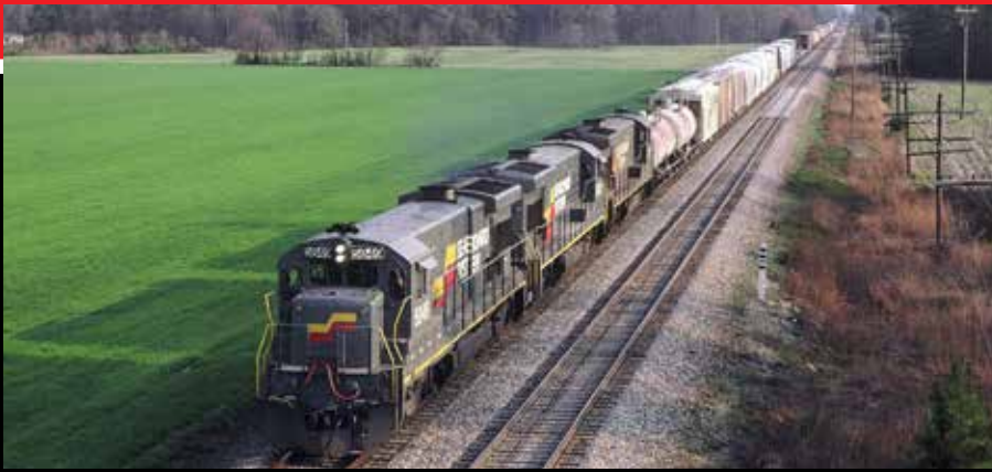
1980-1985 GE B36-7 DC high-adhesion units with solid-state controls
