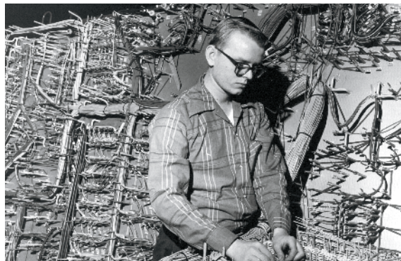
▲ EXANE WIRING There are miles of wire inside a diesel locomotive. Being better suited to the locomotive environment, Exane wire extended running life to more than 50 years.
