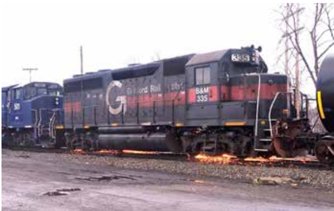
▲ WHEEL CREEP A Pan Am Railway GP40 loses its footing at a higher speed, causing a shower of sparks. The slippage could damage the traction motors, wheel, or the rail. One way to decrease wheel creep is with high-adhesion trucks. Union Pacific No. 5335, a General Electric ES44AC, rides on Hi-Ad trucks introduced with the Dash 9 series in the early 1990s. Left, Robert A. Stein; right, Jeff Wilson
