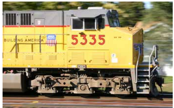
▲ WHEEL CREEP A Pan Am Railway GP40 loses its footing at a higher speed, causing a shower of sparks. The slippage could damage the traction motors, wheel, or the rail. One way to decrease wheel creep is with high-adhesion trucks. Union Pacific No. 5335, a General Electric ES44AC, rides on Hi-Ad trucks introduced with the Dash 9 series in the early 1990s. Left, Robert A. Stein; right, Jeff Wilson
