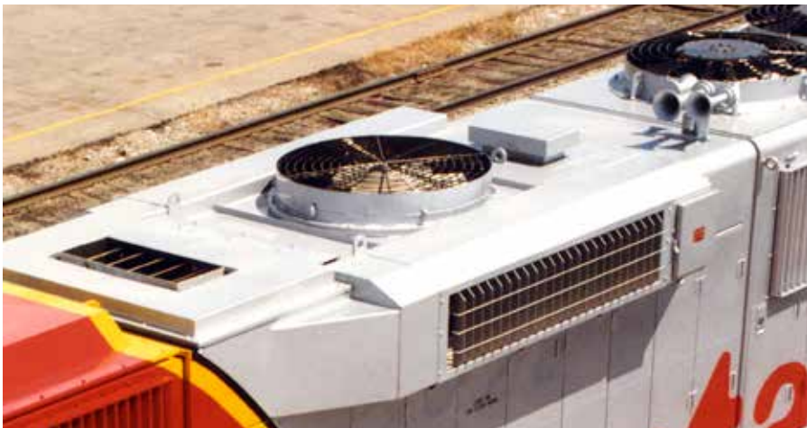
▲ DYNAMIC BRAKE The electric energy created by dynamic braking is dissipated as heat from resistors via the large fan (center) atop the locomotive. This is a new EMD GP60 in 1990. EMD
