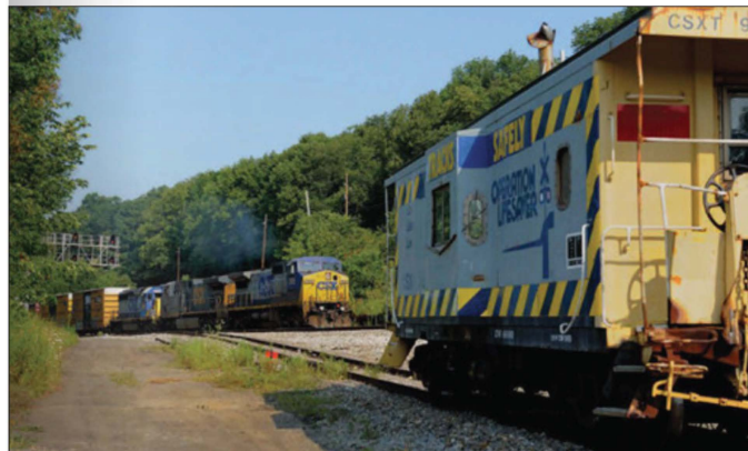
LEFT: The Salisbury Industrial Track connects to the mainline at Salisbury Junction and is the site for some interesting train movements. Because trains run in reverse all the way to the mine, this caboose is left here so the conductor has a safe place to stand while he protects the back-up move across multiple crossings. BELOW: Falls Cut Tunnel is located between two bridges that span Wills Creek and will cross it four more times before arriving in Glencoe. CSX 7352 and his train are making good time heading east towards Fairhope. STAN TRZONIEC PHOTOS
