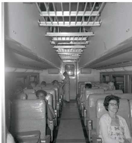
Car 600 interior coach section shows bilevel gallery type seating with reclining seats. Jim Scribbins, Milwaukee Road Historical Association collection
