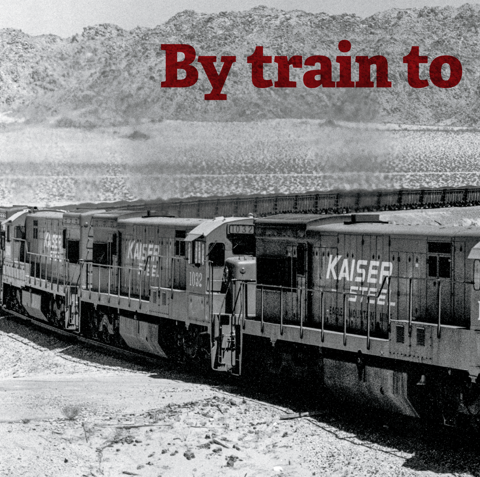
Kaiser Steel's Eagle Mountain Railroad at its zenith in the mid 1970s: bright red U30Cs built to SP specifications leading an endless string of iron ore cars in the Southern California desert.
