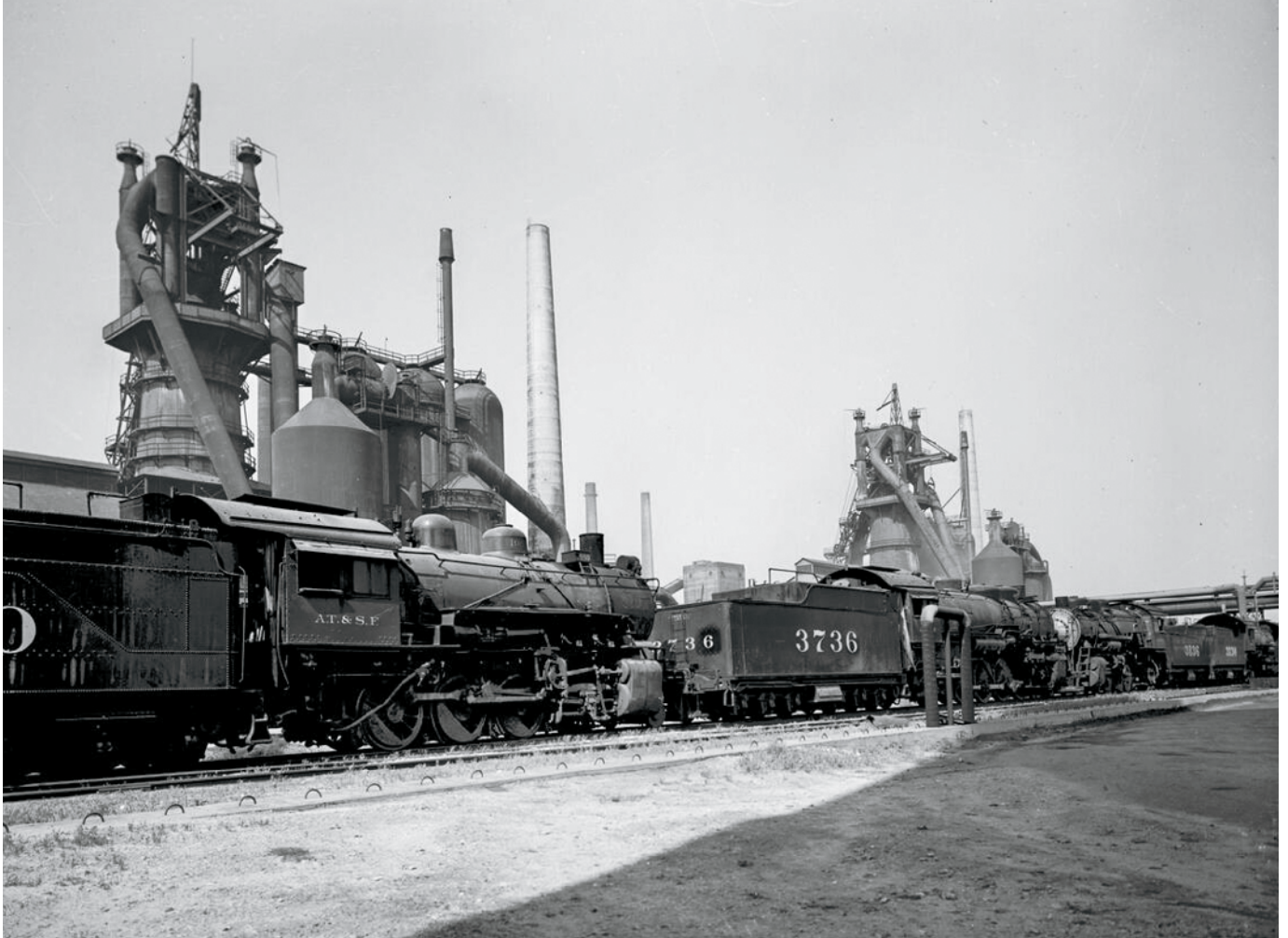
The massive Kaiser Steel complex in Fontana, Calif., was served by Santa Fe and Southern Pacific trackage. Here a row of AT&SF steam locomotives rest beside the mill's blast furnaces in 1952. Kaiser would occasionally rent or lease Santa Fe locomotives for static steam generation at its in-plant power house. Upon retirement, several locomotives were also scrapped on site at the steel mill. USC Digital Library, Los Angeles
