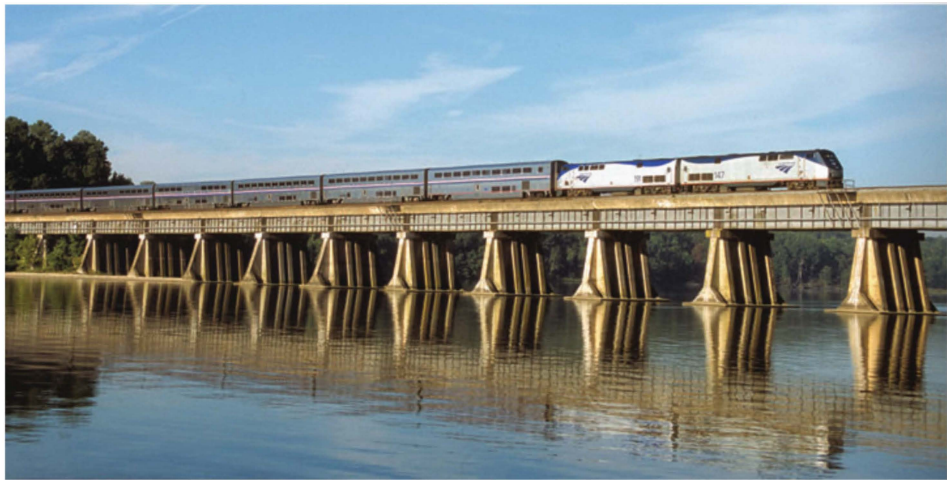
ABOVE: Amtrak's Auto Train at Dumfries, Va., 13 miles south of the Lorton terminal. Two locomotives are standard for the three-quarter-mile-long train, given the relatively flat territory on the route between Virginia and Florida. AMTRAK
