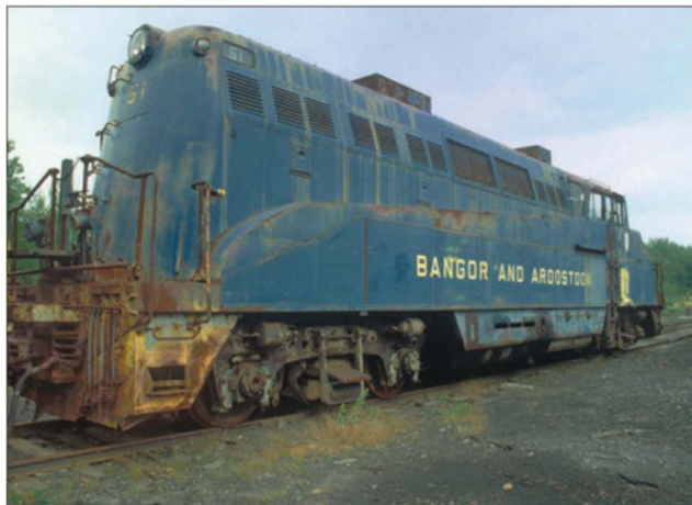
ABOVE LEFT: A full profile from the side shows EMD's early attempt to make a dual purpose locomotive. Both sides have been somewhat relieved of sheet metal with extra windows in the cab facing rearward for switching or transfer moves. BAR 51 was discovered in repose on the dead line in 1989. ABOVE RIGHT: Basic steps and footboards were the hallmark of the early diesels. Take note of the inside depth of the steps allowing for plenty of footwear room even in the nastiest of winter weather conditions in northern Maine. RIGHT: From the rear of the engine compartment, the standard EMD 567B prime mover is indeed impressive. Quarters are tight but using a very wide angle lens makes it look like there is plenty of room for maintenance on this 1500 h.p. V16 engine. Steps lead to the cab; the back of the engineer's chair can be seen through the door.
