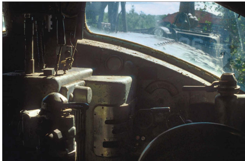
LEFT: The BL2 has many elements reminiscent of the popular F3 cab unit that preceded it, such as the unique forward window shape and cab contours. Snow brooms were standard issue for BAR locomotives, note the dedicated receptacle. BELOW: Looking up and out towards the front of the BL2, one takes note of the short hood through the automotive styled windshield. Horn controls are to the left; one for the front, one for the rear facing horn. Built as 551 in 1949, it was renumbered 51 in 1953, and scrapped in 1993.
