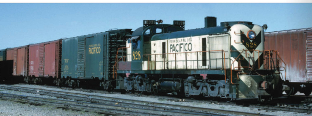
ABOVE: The first diesels on FCP were RSD-5s, with 35 purchased in just over two years. Crisp cream and green paint is displayed on 828 on February 12, 1965, at Hermosillo, Sonora. The entire fleet was equipped with m.u. and dynamic brakes, and they were the only diesels until S-6 deliveries started in 1955.
