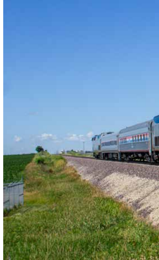
A northbound test train approaches the Airport Road grade crossing north of Springfield, Ill., at 90 mph on June 25, 2020. Technicians in the bungalow are monitoring track circuit and IETMS/XITCS data; flaggers (not visible) protect the crossing. Bob Johnston
