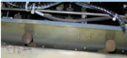
Two spikes inserted below Lockheed Martin's Location Determination System reduced vibration. Daniel L. Steinhoff
