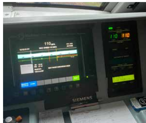
A Siemens Charger shows IETMS positive train control and XITCS displays during current 110-mph operation. XITCS status information is in the gray block at the left center of the PTC screen. Greg Richardson
