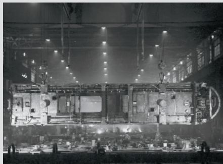
2 A piped and cabled underframe is lifted for positioning in the assembly area.
