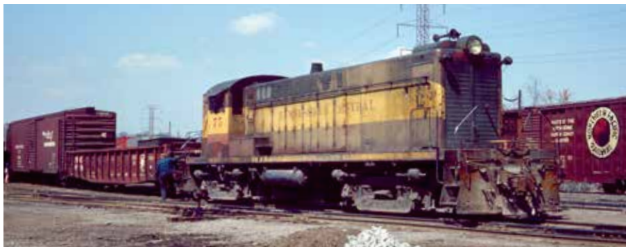
TC Nos. 75–77 were Baldwin's first DRS-4-4-1000 road-switchers, predating a demonstrator. No. 75 works in Nashville's Southern Junction Yard, TC's hub, in April '66. They served 18 years.
