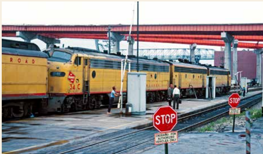
About an hour later, MILW's Chicago-Minneapolis Morning Hiawatha takes on fuel and changes crews during its Milwaukee stop. FP7 100A and E9 34C sandwich an F7B.
