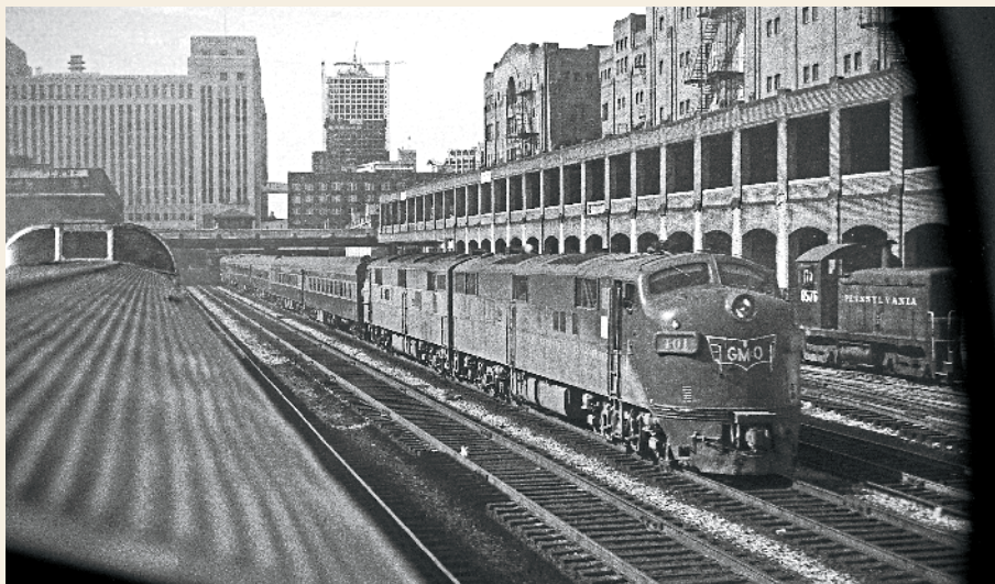
A rearward view from a dome on BN's Afternoon Zephyr shows Gulf, Mobile & Ohio E7s shoving the Abraham Lincoln toward Chicago Union Station before its afternoon departure for St. Louis on June 5, 1970. At right is the former PRR Polk Street Freight House and an ex-PRR SW1.
