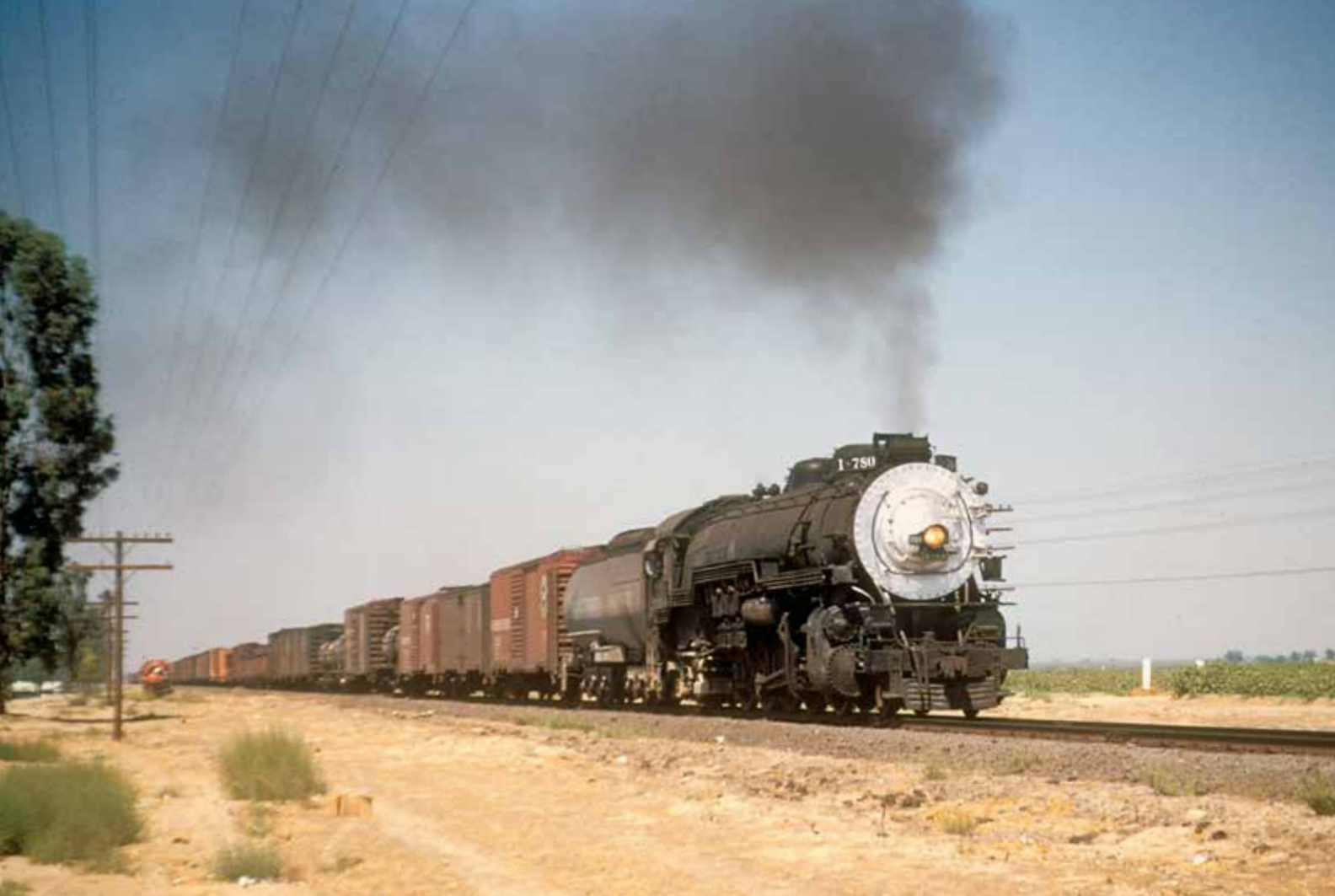
The “1-780” in the train indicator boards flanking the smokestack of SP 2-10-2 No. 3744 show that this is the first section of eastbound freight train 780, pictured near Traver, Calif., on September 5, 1953. If this were a nonscheduled “extra” train, the indicators would display “X3744.”
