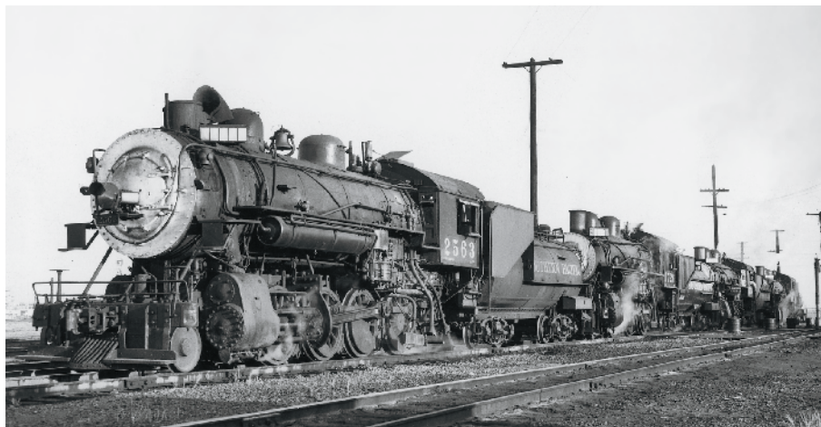
Engines for San Joaquin Division local trains await their morning runs at Fresno in mid-1956. Considered big power when they were built in the first decade of the 20th century, Consolidation 2563 and Moguls 1726, 1774, and 1727 remain useful for light work five decades later.
