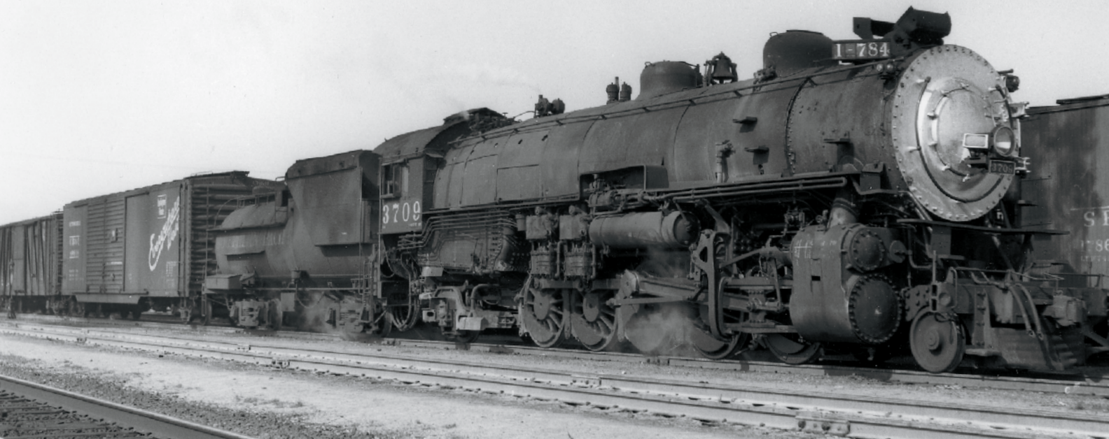
SP relied heavily on 117 63-inch-drivered 2-10-2s of classes F-3, F-4, and F-5 built by Baldwin during 1921–24. The “F” was derived from “Freight”; crews called the 10-coupled engines “Decks” (from “Decapods”). F-4 No. 3709 departs Fresno with First 780 in February 1952.
