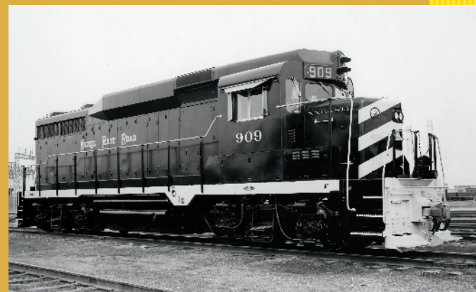
Nickel Plate 909 poses for its builder's photo. Like ACL and NYC, NKP opted for units without dynamic brakes. EMD
