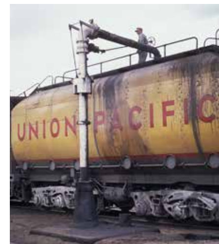
A hostler fills the tender of GTTEL No. 25 with Bunker C oil. GTTEs Nos. 1-30 were mated with modified tenders from retired 4-8-4s.
