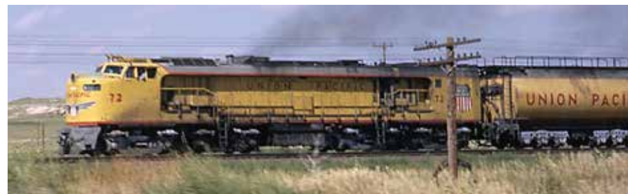
After buying GE's 1948 GTTEL prototype, a single-unit B-B+B-B, UP ordered 25 similar units, delivered in 1954. Some, like No. 72, westbound at Potter, Nebr., had exterior side walkways.
