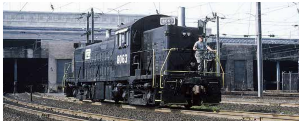
Lima-Hamilton built PC 8063 for NYC, which gave it an EMD engine in 1957. A boiler in the short hood won it and sister 8062 coachyard jobs at Chicago, then Philly, where it works in June '69.
