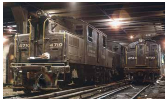
The oldest units on the PC roster were the S motors, built during 1904–08 for NYC's third-rail lines into Grand Central Terminal. Long since demoted to switching duty, three rest under GCT in March '72.
