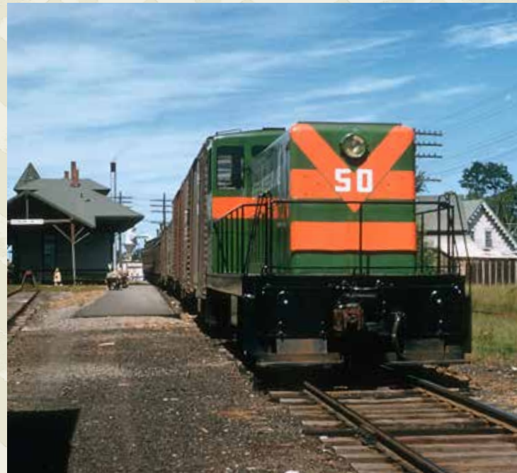
Exhibiting the original 70-tonner front end — round headlight casing and solid nose — Belfast & Moosehead Lake No. 50 is at Burnham Junction, Maine, in July 1957. Soon she'll leave the depot, shared with Maine Central, with a mixed train for Belfast.
