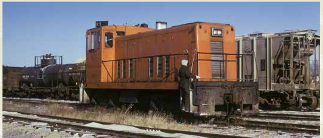
The most common 70-tonner face — a rectangular twin headlight casing above a louvered radiator intake — was introduced in September 1949. Iowa Terminal Railway 76, built for WP subsidiary Tidewater Southern, is at Charles City in January '76.
