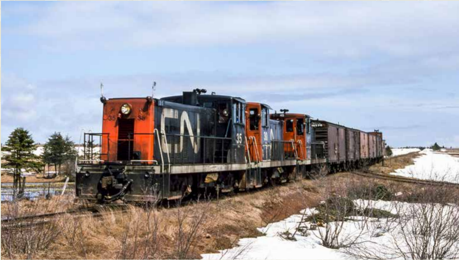
Canadian National received 18 70-tonners for its Prince Edward Island lines in the first half of 1950. The road apparently preferred the old-style headlight over the new twin-bulb type. Three units trundle east with five empty reefers for potato loading at Souris, P.E.I., on April 28, 1975.
