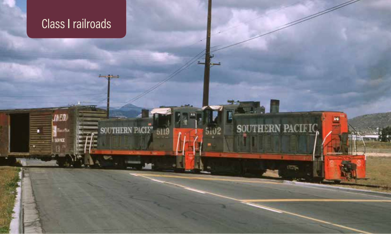
Southern Pacific had the biggest fleet of 70-tonners in North America, buying 21 during 1949–55. Many worked in Oregon and Arizona; others went to subsidiary San Diego & Arizona Eastern. Engines 5102 and 5119 are at the end of the SD&AE's El Cajon, Calif., branch in February 1964.
