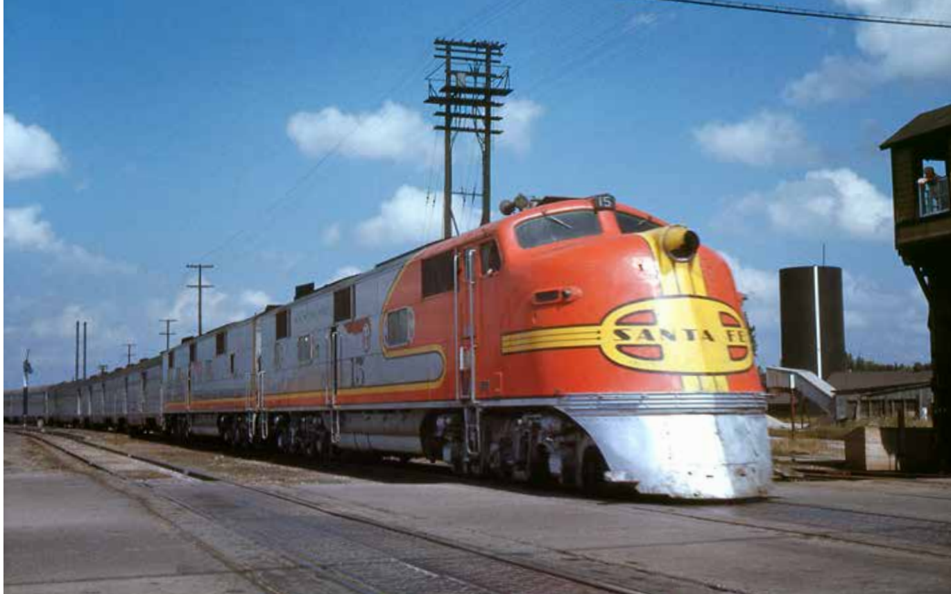
Diesels enabled engine runs unimaginable with steam. In August 1942, E6A No. 15 and a B unit bring the streamlined Chief into Streator, Ill., 90 miles into its 2,227-mile dash to Los Angeles. The hood over the headlight was a requirement for locomotives operating on the Pacific Coast.
