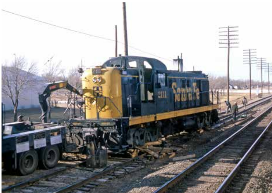
Crews work to rerail Alco RSD5 2111, which apparently had an earlier incident while working at Pampa, Texas, prior to Dave's train passing it on December 27.
