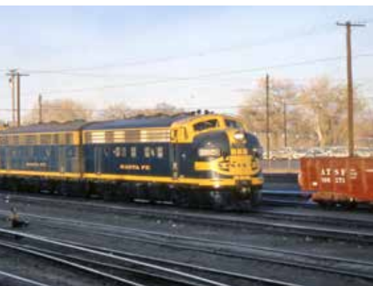
Baldwin DS-4-4-10 2295 works at Clovis, N.Mex., on December 27. The unit's single stack shows it to be a six-cylinder turbo-charged variant. The railroad had 41 such units, along with 59 V01000s and a single V0660, the former demonstrator 62000.
