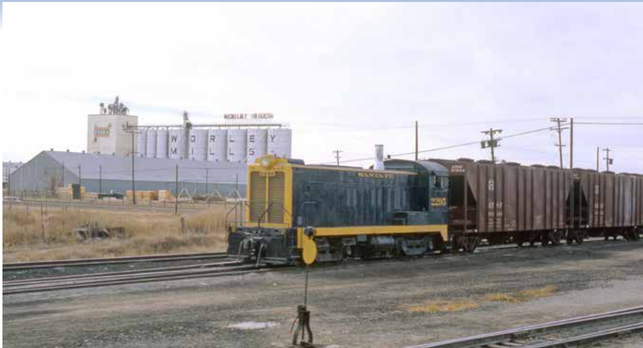
Baldwin DS-4-4-10 2295 works at Clovis, N.Mex., on December 27. The unit's single stack shows it to be a six-cylinder turbo-charged variant. The railroad had 41 such units, along with 59 V01000s and a single V0660, the former demonstrator 62000.
