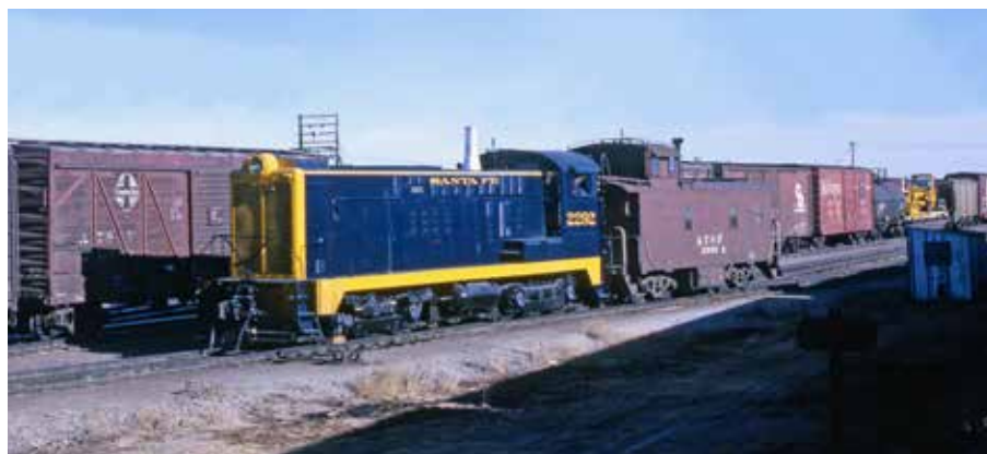
Another DS-4-4-10, 2292, works in the sun at Vaughn, with a trademark Santa Fe cupola caboose. The caboose number, 2089R, indicates that the car is radio-equipped.
