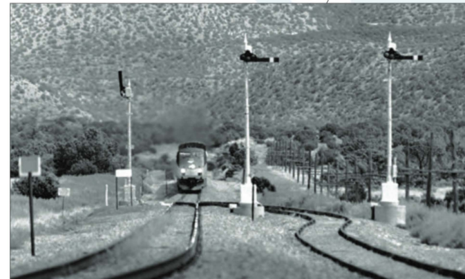
OPPOSITE TOP: Rolling toward the landmark bulk of 7,031-foot Starvation Peak on Tuesday, October 13, 2020, Amtrak Train 3 encounters high green at the east end of Chapelle. Some 22 signals at nine installations between mileposts 774 and 791 comprised the last stand of semaphores on the Glorieta Subdivision.
