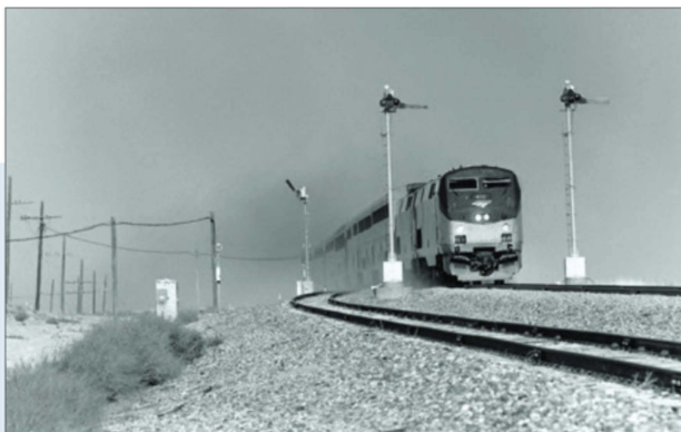
ABOVE: Following a round of signal replacements in 2015, the east end of Wagon Mound siding marked the western boundary of semaphores on the Raton Subdivision — 20 signals in eight installations between mileposts 706 and 725. Thursday, October 8, 2020, finds westbound Train 3 approaching the east switch at Wagon Mound behind a trio of P42DCs.
