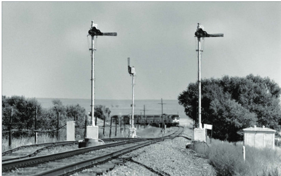
ABOVE: Following a round of signal replacements in 2015, the east end of Wagon Mound siding marked the western boundary of semaphores on the Raton Subdivision — 20 signals in eight installations between mileposts 706 and 725. Thursday, October 8, 2020, finds westbound Train 3 approaching the east switch at Wagon Mound behind a trio of P42DCs.
