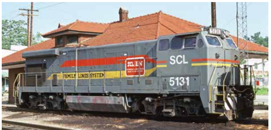
SCL's GP16 program rebuilt 155 old GP7s and 9s into virtually new locomotives during 1979–82; GP16 4700 leads two other units at Atlanta in May 1981 (left). SCL was the only buyer of GE's "crew quarters" cab BQ23-7; "Q-boat" 5131 is at Lawrenceville, Ga., in June '82 (above).
