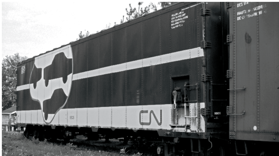
Both passenger and freight versions of CN's auto carriers were spotted at Drummondville, Quebec, in 1993. Built in 1957 by Canadian Car & Foundry, each 56-foot, double-deck, double-ended-door car could accommodate six automobiles.
