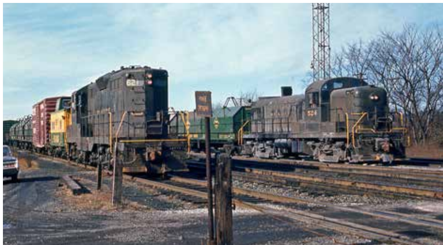
EMD GP7 621 and Alco RS3 524, working at Abrams Yard near Norristown on January 7, 1972, represent the most common first-generation power used on Bee-Line trains. The 621 survives in the Reading Company Technical & Historical Society collection at Hamburg, Pa.
