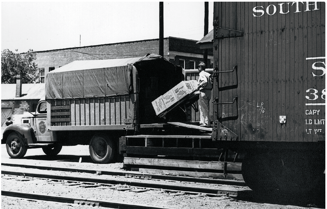
Railroads used trucks to expand their services. Here, cases of cereal are transloaded from a boxcar to a truck of Cotton Belt subsidiary Southwestern Transportation for local delivery. As less-than-carload shipments became unprofitable, railroads ceded such traffic to motor carriers.
