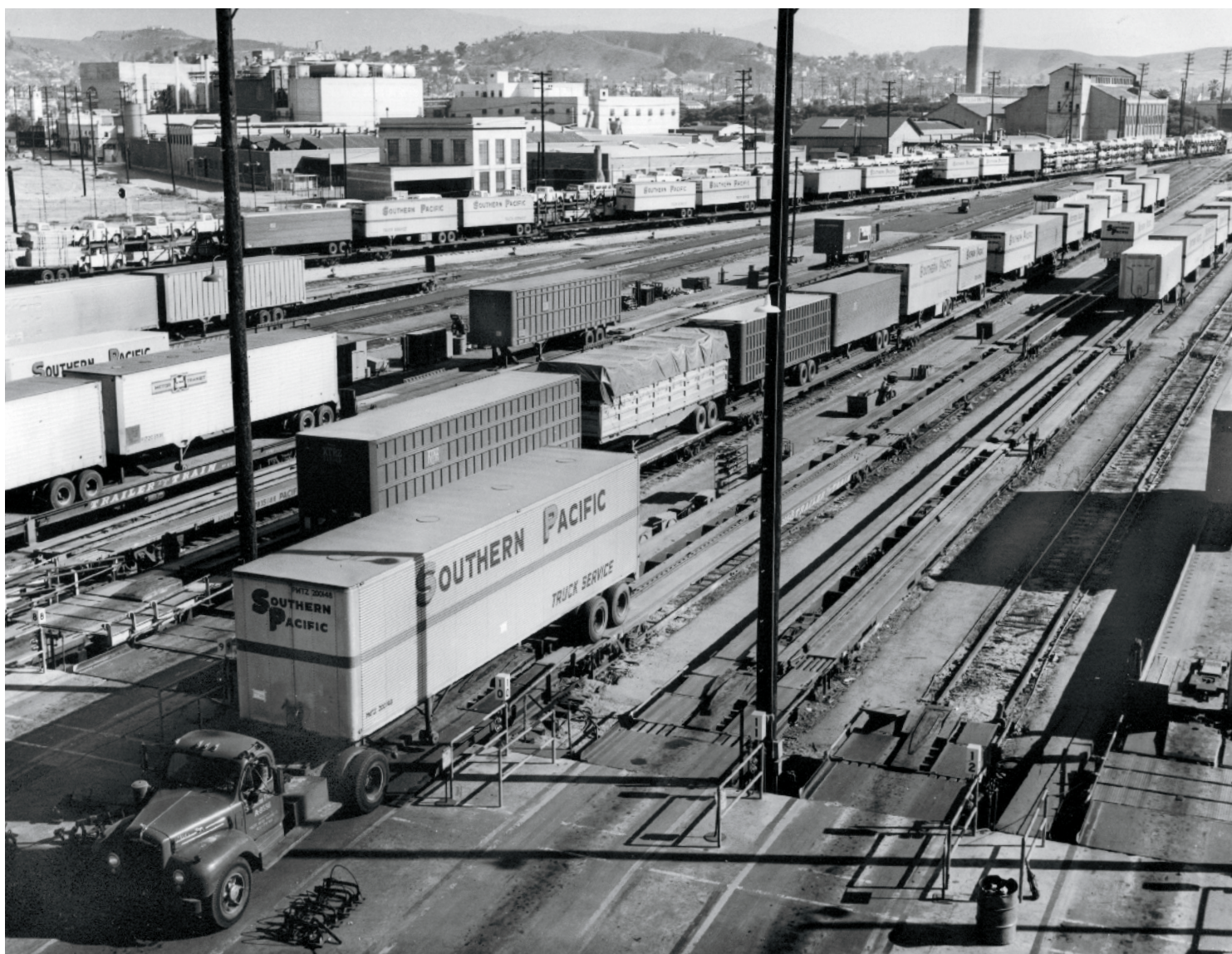
Railroads have found prosperity in the highway age by hauling truck trailers and containers on flatcars. Multi-level auto-rack cars, like those in the background of this early 1960s Southern Pacific scene, enabled the rails to recapture lucrative finished-vehicle traffic from truckers.
