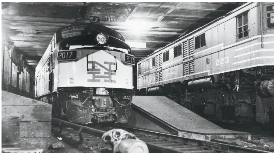
When the FL9s were new, TRAINS Editor David P. Morgan enthused about their "bringing the modern era" into Grand Central Terminal, wonderfully illustrated in comparing 2017 next to the heavily riveted New York Central P-2b class box-cab electric 223 on February 10, 1958.
