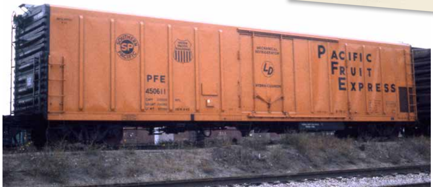
Above: Mechanical reefers grew larger in the 1960s, as shown by Pacific Fruit Express No. 450611. The 57-foot, exterior-post car was built in 1963. J. David Ingles collection Inset: An excerpt from a Rock Island brochure extolling the new mainline icing plant in the 1950s. CLASSIC TRAINS collection
