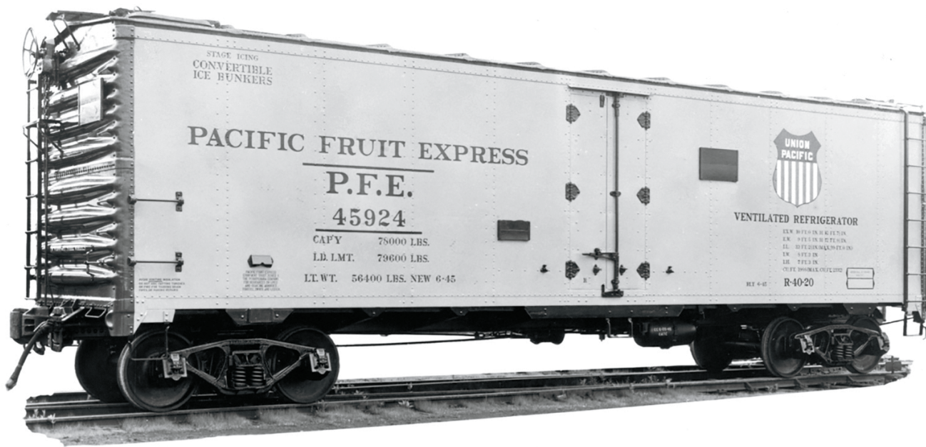
Pacific Fruit Express acquired 1,000 R-40-20 reefers in 1945. The 40-foot steel cars had 4/4 Dreadnaught ends and featured improved (fiber-glass) insulation and floor racks. Later paint schemes had both Southern Pacific and Union Pacific heralds. Union Pacific
