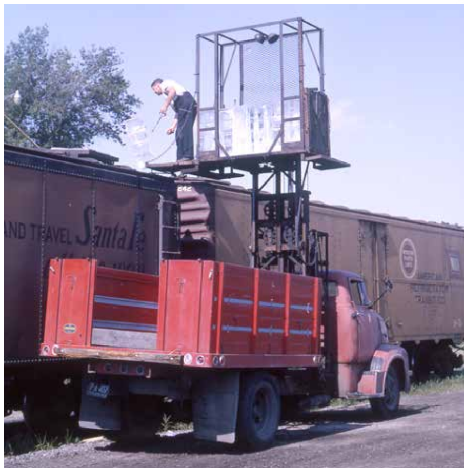
Above: Small heaters would keep loads from freezing in cold weather. Early models were charcoal-fueled and later ones ran on alcohol. CLASSIC TRAINS collection Left: A local ice contractor with a hoist truck tops off the bunkers of Santa Fe and ART reefers parked on a spur in Ohio in 1964. J. David Ingles collection
