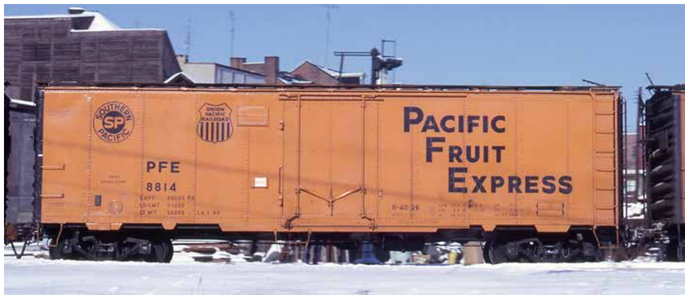
Sliding plug doors began to replace swinging doors around 1950. PFE's 2,000 R-40-26 cars were built in 1951 and 1952. Ice reefers were also used in ventilator service, which saw the roof hatches opened to enable air to flow through the cars. J. David Ingles collection
