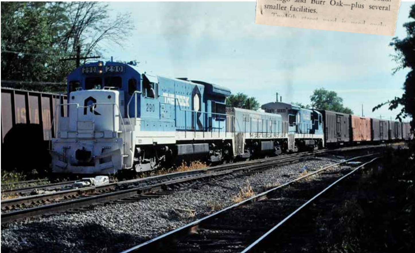
A U33B-slug-U33B set in the Rock's late "bankruptcy blue" scheme has a block of reefers in tow at Bureau, Ill., in 1978. The lettering on the side of the slug dubs it "The Great American Energy Saver," a nod to the newfound energy conservation movement of the decade. Mark Llanuza
