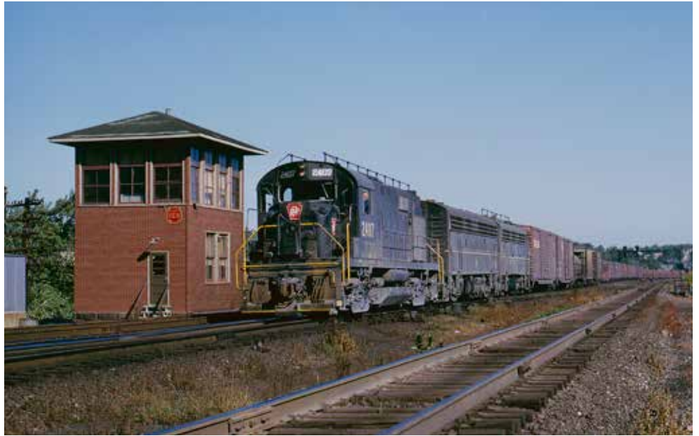
At Duncannon, Pa., near the east end of PRR's Harrisburg-Pittsburgh main line, an Alco RS27 and two F units lead tonnage east past View tower, whose operators looked out on a sweeping panorama of the Susquehanna River valley. The first and third units carry antennas for PRR's Trainphone communication system; the largest rail user by far, PRR retired the system in favor of conventional radio two years after this 1964 photo.
