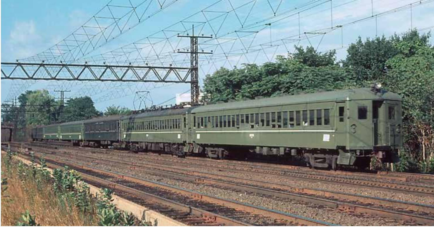
Penn Central inherited a number of NH's ancient trailer-motor-trailer M.U. sets, two of which (in NH and PC greens) roll east under triangular catenary at Port Chester, N.Y., in August 1970. The legions of commuters who depended on PC ensured that the road's troubles were acutely felt by a wide public. George Krambles, Krambles-Peterson Archive
