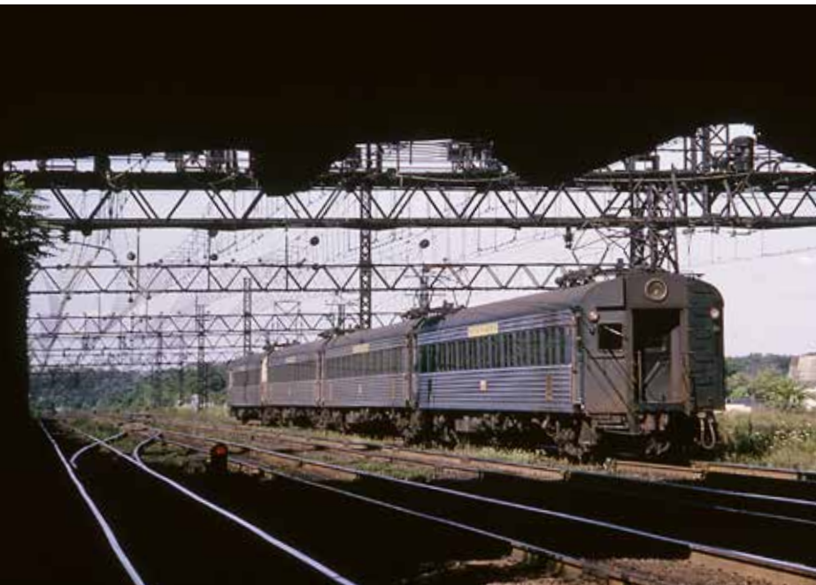
Four New Haven "Washboard" M.U. cars pull away from the station at Rye, N.Y., in July 1965; traveling under a web of wires here, the train began its run on third-rail power at Grand Central Terminal. Pullman-Standard built 100 such cars at its Worcester, Mass., plant in 1954; they replaced 150 cars from the early years of NH's electrification, which began in 1907.
