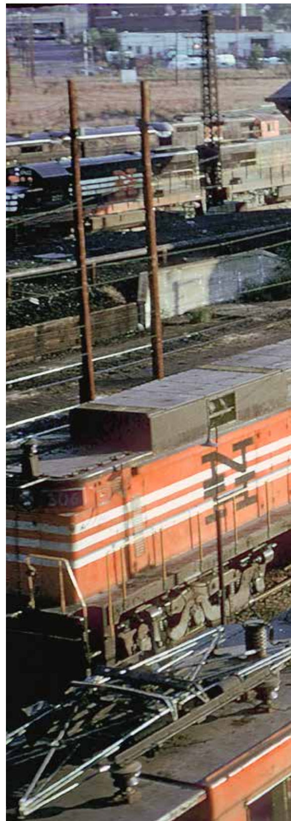
Four New Haven "Washboard" M.U. cars pull away from the station at Rye, N.Y., in July 1965; traveling under a web of wires here, the train began its run on third-rail power at Grand Central Terminal. Pullman-Standard built 100 such cars at its Worcester, Mass., plant in 1954; they replaced 150 cars from the early years of NH's electrification, which began in 1907.
