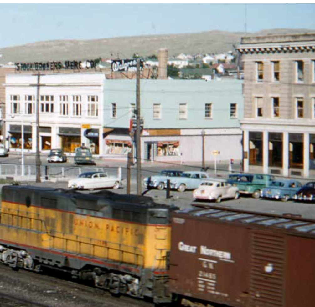
ROCK SPRINGS, WYOMING: Union Pacific bought more cabless road-switchers than any other carrier. The big road's enthusiasm for B units is on view at Rock Springs, Wyo., where a GP9 and three GP9Bs hustle a freight east past the depot and downtown buildings in the 1950s.
