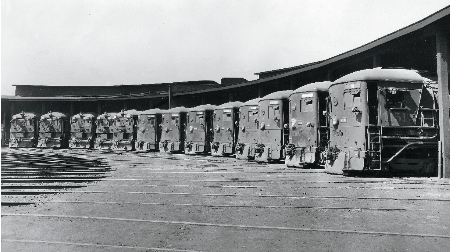
ROSEVILLE, CALIFORNIA: Sometime in the late '30s, 13 cab-forward 4-8-8-2s look out from the roundhouse at Roseville, junction of the Overland Route with a line to Oregon and site of a major freight yard. A response to Donner's snowsheds, cab-forwards came to SP in 1909; the road had more than 250. Southern Pacific
