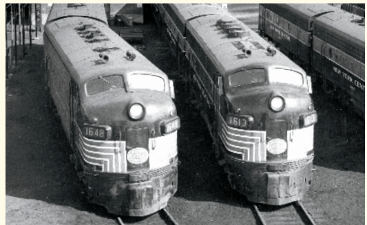
F3 vs. F7: F3s (and F2s) with dynamic brakes had two rectangular openings aft of the air horns (right above); on F7s and F9s with dynamics there was a fan (left). Units without dynamics had plain sheet metal there.
