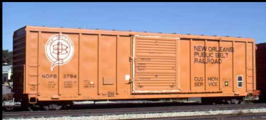
→ New Orleans Public Belt was a major operator of IPD cars, with 1,100 by 1981. This Plate C car was built by Pullman-Standard in February 1979 and financed by Itel Rail.
