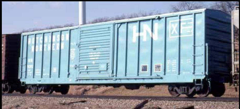
→ Hutchinson & Northern's entire 575-car roster was made up of IPD boxcars, including 325 class XF food service cars. Note the "XF Food Loading Only" lettering at right on No. 5082, built by Mexican builder CNCF in July 1979 and photographed in 1980. J. David Ingles
