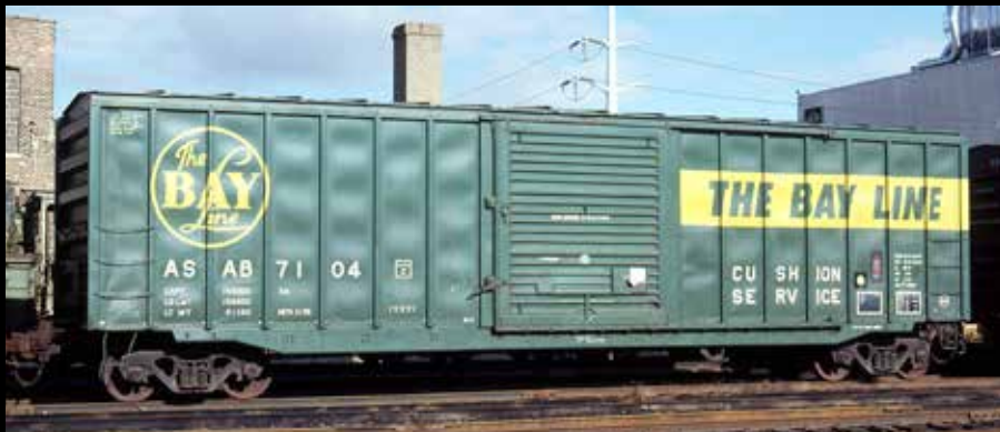
← Atlanta & St. Andrews Bay eventually acquired 300 IPD boxcars. Number 7104, a 5,300-cubic-foot Plate C car, was built by ACF in November 1976 and photographed in November 1978.
