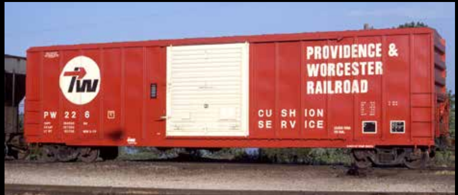
→ Providence & Worcester No. 226 is a Plate C car built in February 1977 by FMC in Portland, Ore.; it's shown in July 1977. The railroad had about 600 IPD cars on its roster, financed by SSI (note the "Leased from SSI Rail" stencil). R. J. Wilhelm, J. David Ingles collection
