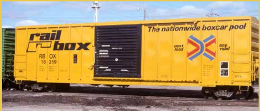
This Railbox Plate B car was built by FMC in November 1975. Although colorful and featuring the same basic design as many IPD cars, Railbox cars did not qualify for incentive rates. R. J. Wilhelm, J. David Ingles collection
