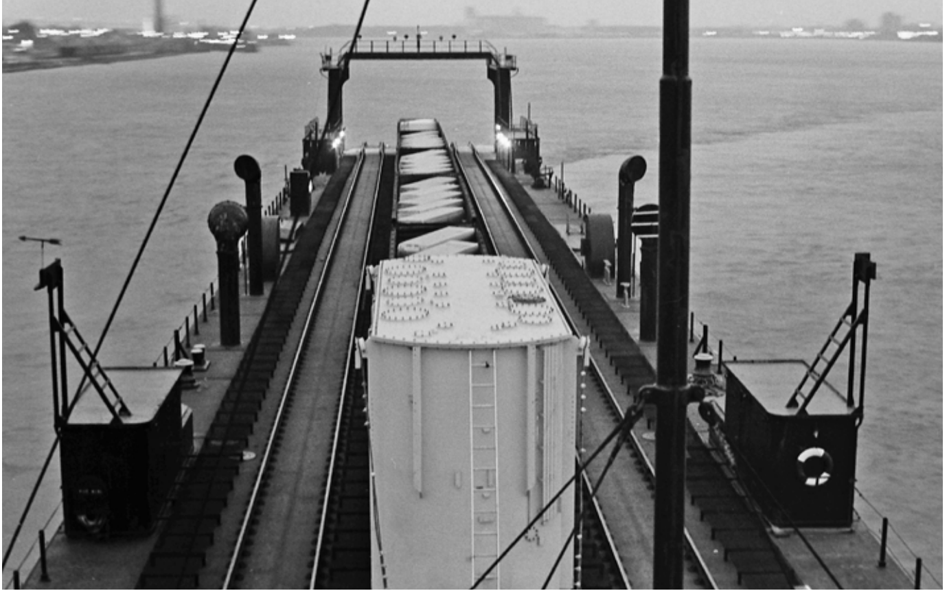
The gondolas with aluminum ingots and the transformer are the only loads for CN's barge St. Clair as it is pushed by the tug Phyllis Yorke across the St. Clair River to Port Huron, Mich., "sneaking" me back into the U.S. CN kept the carferry service as a St. Clair Tunnel bypass.
