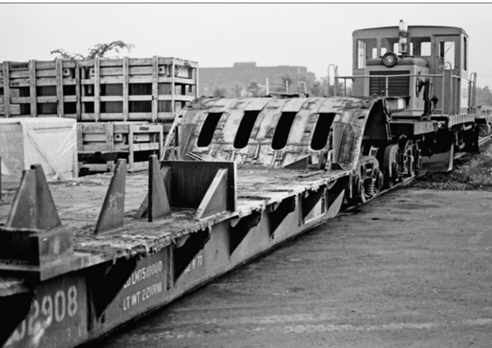
The GE 45-tonner at ASEA's Varennes plant hostiles empty N&W drop-center flatcar 202908, which CN has spotted for loading. Before the transformer can be put aboard, though, major deck-cleaning is necessary. After it's loaded, the GE will flap its siderods to come retrieve it.
