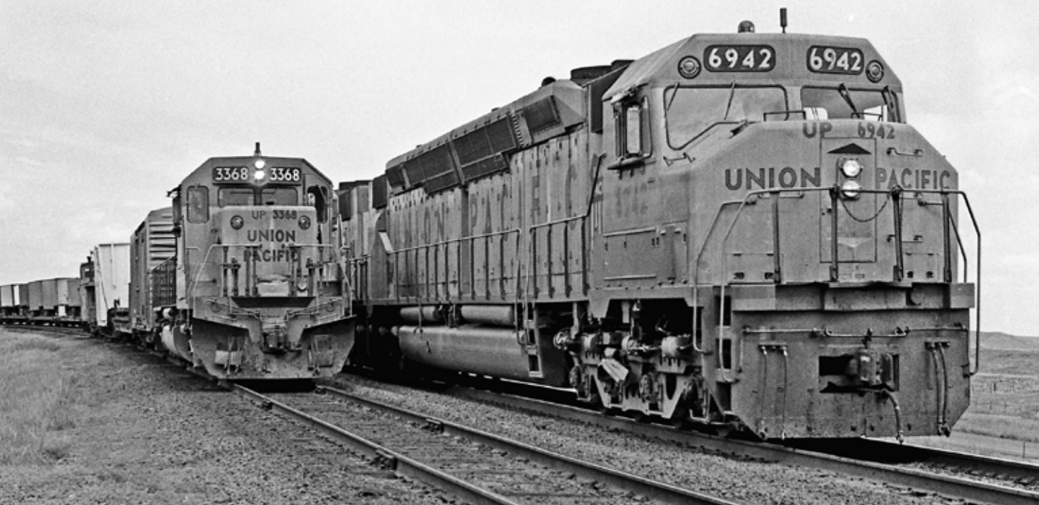
On Union Pacific, most of the hot freights that passed us in either direction were led by twin-engined DDA40X Centennial units, as here near Laramie, Wyo. Crews hated working our 35-mph train, as with each passing westbound, another crew in their pool was running around them.
