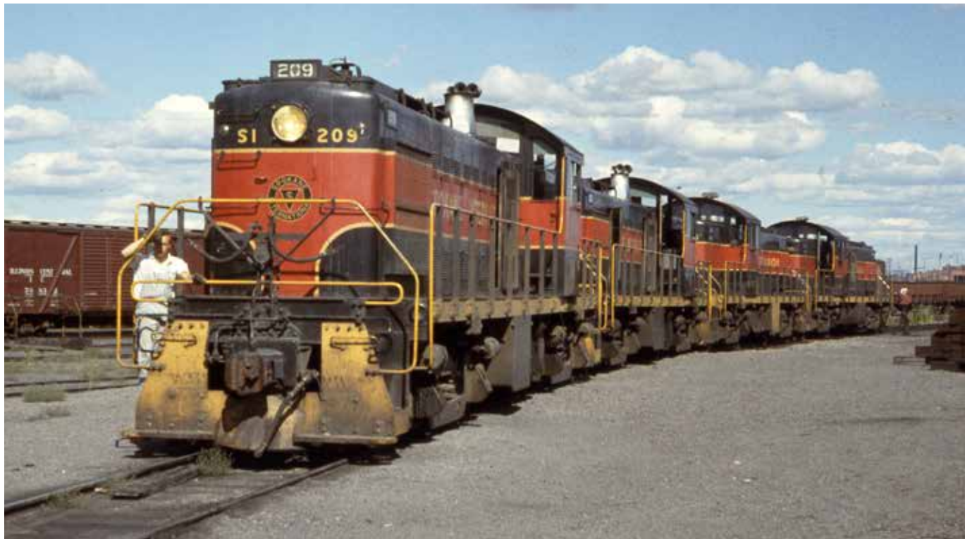
Four of Spokane International's RS1s move in Spokane yard on September 3, 1956. All 12 were equipped to run in multiple, and did so regularly.
