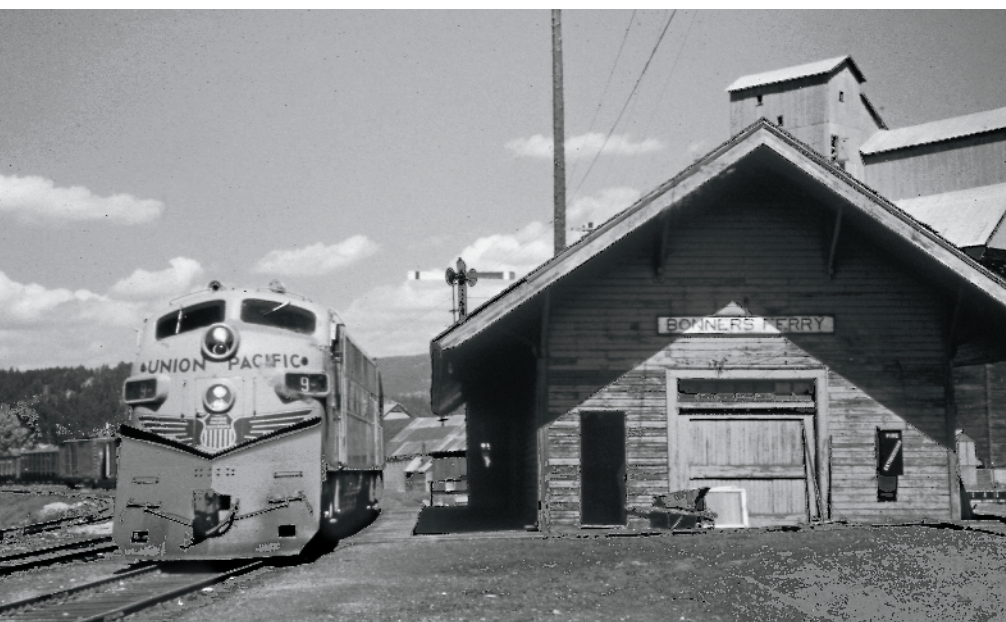
On August 6, 1961, Eastport–Spokane through freight No. 9 is at Bonners Ferry, Idaho, its locomotives — UP F3s rebuilt into F9s — reflecting the shift from RS1s as road power on SI.
