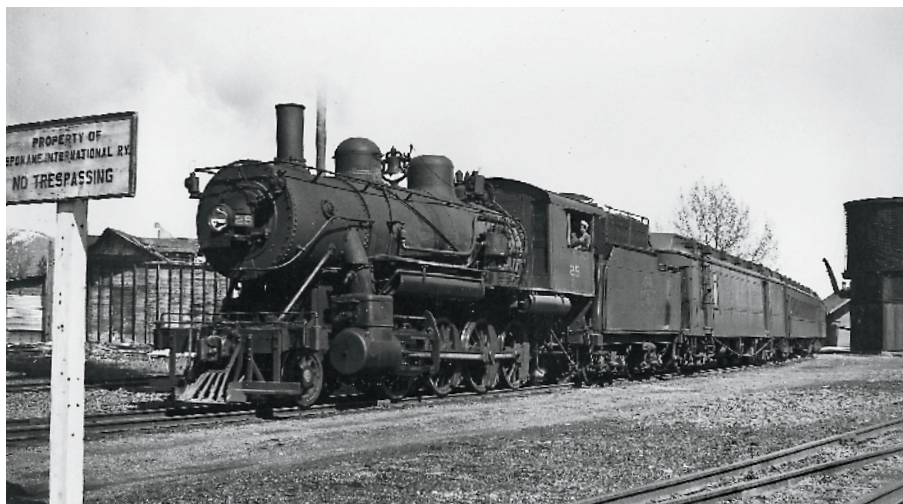
Fireman Bill Miller leans out the cab window of 2-8-0 25 as train 1 departs Sandpoint, Idaho. L. E. Shawver
