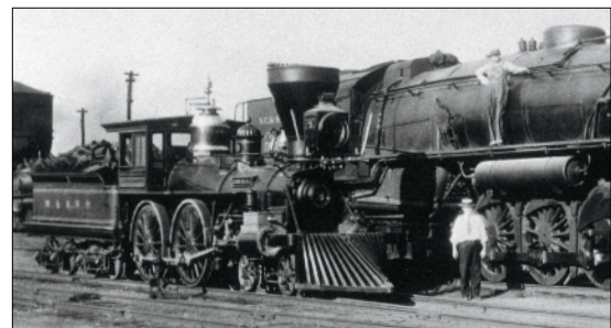
Compare W&A 4-4-0 No. 3, the Civil War-era General , with 565, first of NC’s five J2 class 4-8-4 “Dixies” built at Schenectady in 1930.
