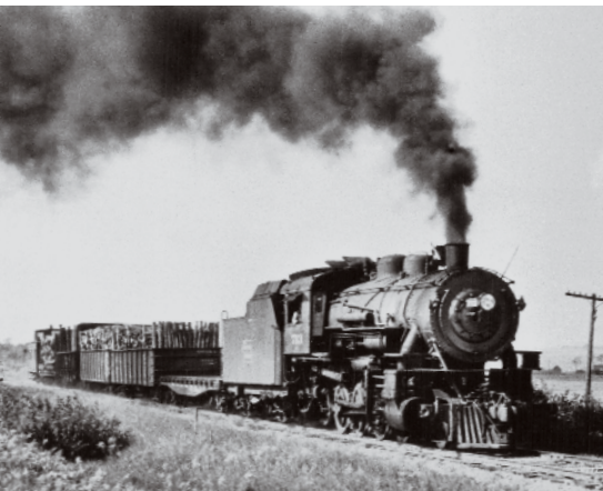
Typical of the DSS&A, 2-8-0 713 hauls a short train on stamp sand ballast near Paynesville.
