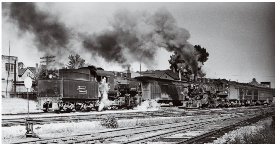
At DSS&A's Marquette station on a September 1951 afternoon, 2-8-0 92 makes up train 7, which will run overnight to Duluth, as 4-6-2 556 pulls out with Mackinaw City-Calumet train 1.
