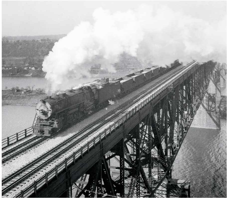
Symbolic of the heavy-haul Bessemer, one of its 47 powerful 2-10-4 Texas types crosses the huge Allegheny River bridge with Minnesota iron ore in October 1934. CLASSIC TRAINS collection
