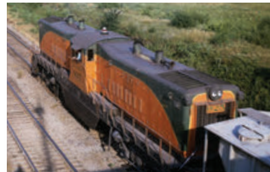
Roof details on EMD-engined “SW2400” (as some fans called J’s rebuilt Baldwin center-cabs) 925 are evident at Brisbane, Ill., in 1965.
