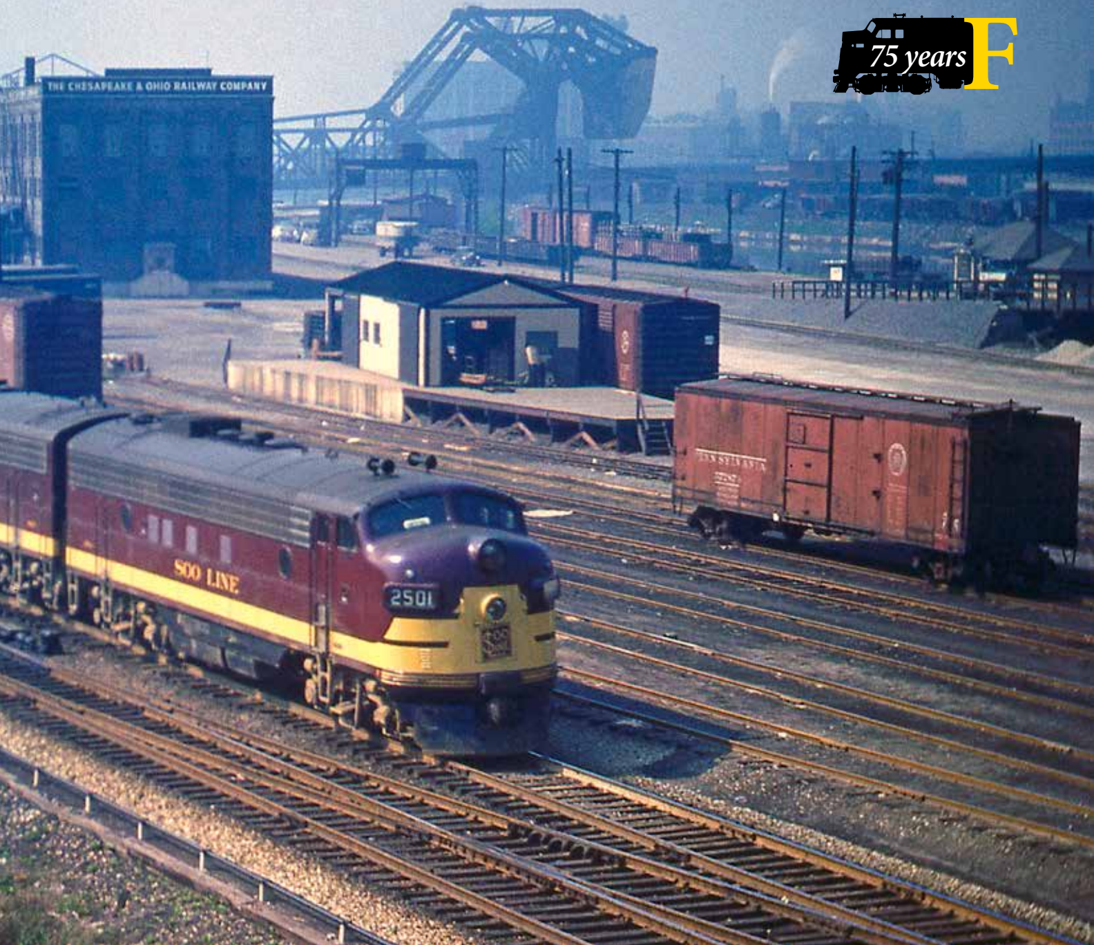
SOO LINE , whose train 18, soon to be named Laker (above), nears Chicago's Grand Central Station in May '51 behind FP7/F7B 2501A&B, was among FP7 owners that ran few passenger trains. GEORGIA 1004 (inset), in Atlanta in late 1966, clearly exhibits the FP7's 4 feet of extra length, behind the forward truck.
