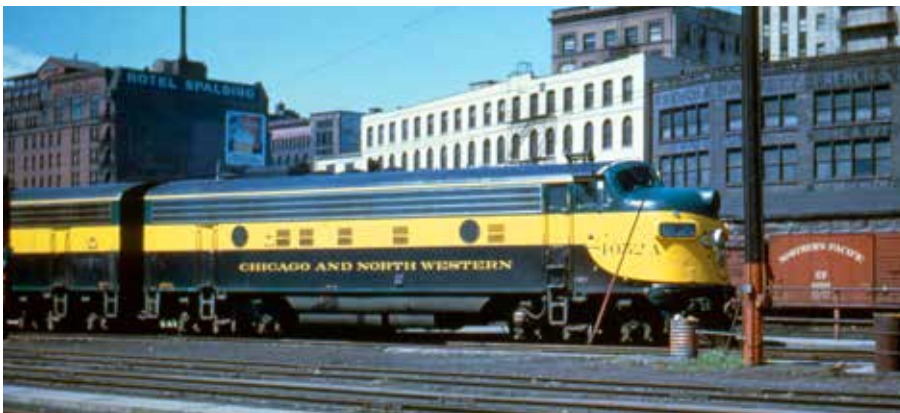
NORTH WESTERN had the only U.S. "FP9s," 1955 FT rebuilds rated at 1,500 h.p. and designated FP9M. Their careers in passenger service, and in this livery (at Duluth), were relatively short.
