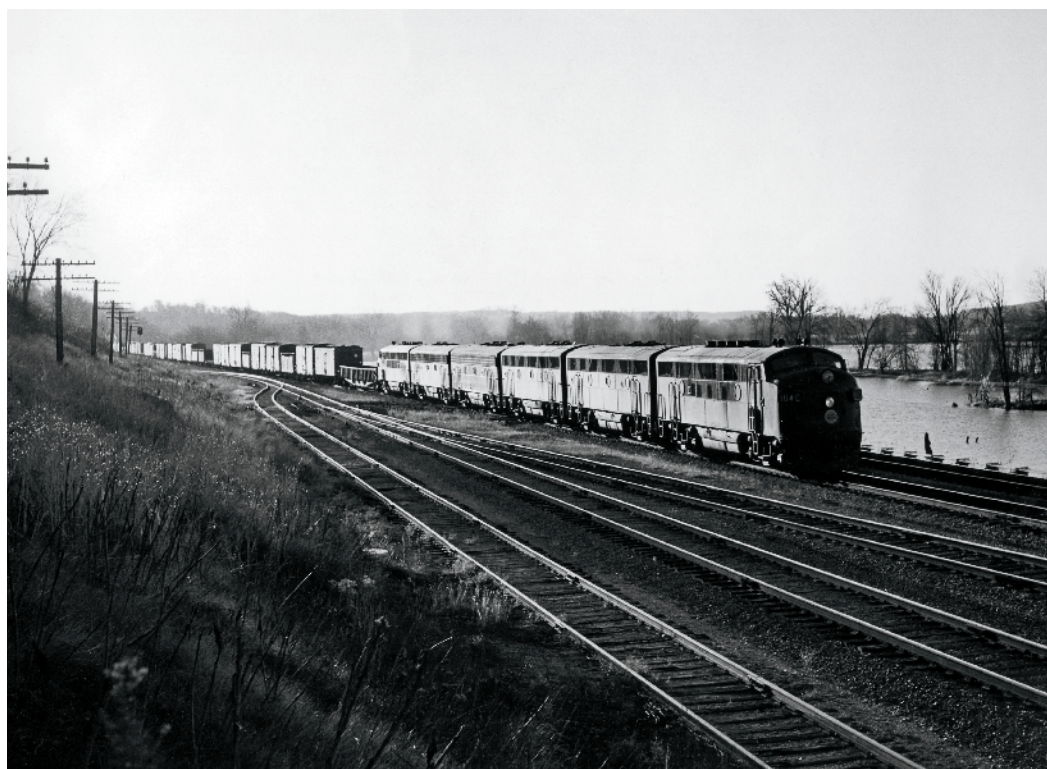
Chicago Great Western was probably most known in dieseldom for running one or two daily huge road freights with five or more F units, as here on 150-car Chicago–Oelwein (Iowa) train 91 at Portage, Ill., on CB&Q trackage rights along the Mississippi River in November 1956. CGW owned 74 Fs: 33 F3As, 16 F3Bs, 4 F7As, 19 F7Bs, and 2 FP7s. The FP7s, 3 F3As, and 4 F7As were passenger units.
