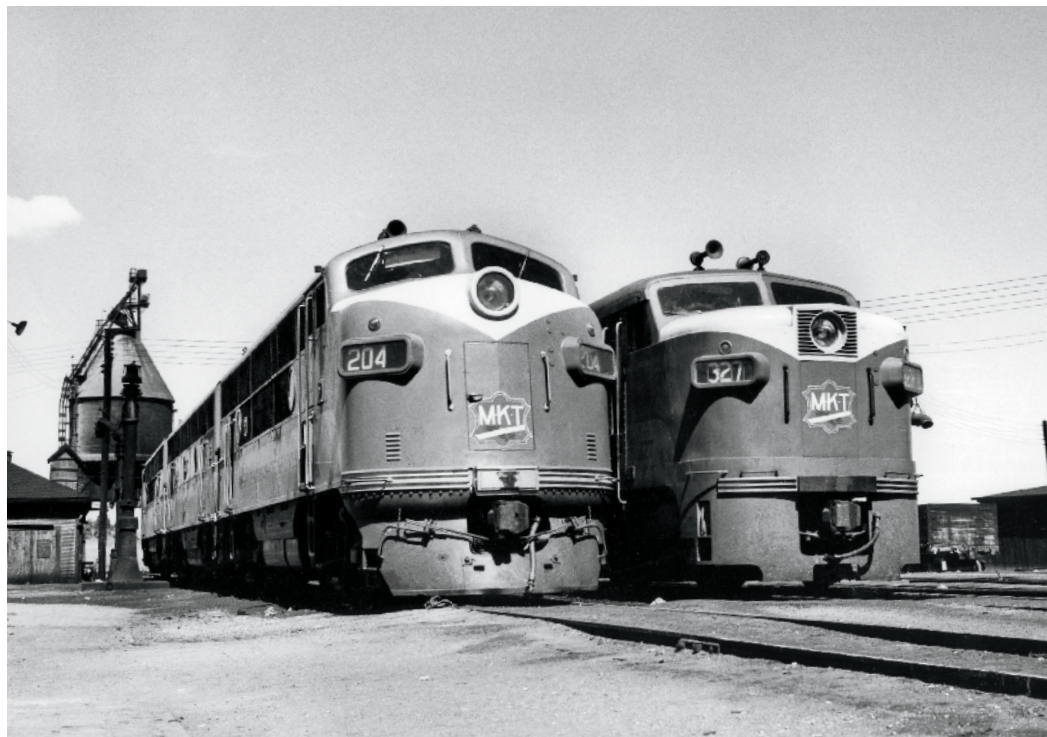
Missouri-Kansas-Texas F3 204 and FA1 327, at Denison, Texas, in 1949, show the contrast in nose design between EMD's rounded "bulldog" and Alco-GE's flatter style. Both sets are in Katy's original red and cream livery. MKT owned 19 FAs and 90 total Fs; 13 FAs were re-engined by EMD in 1956–59.
