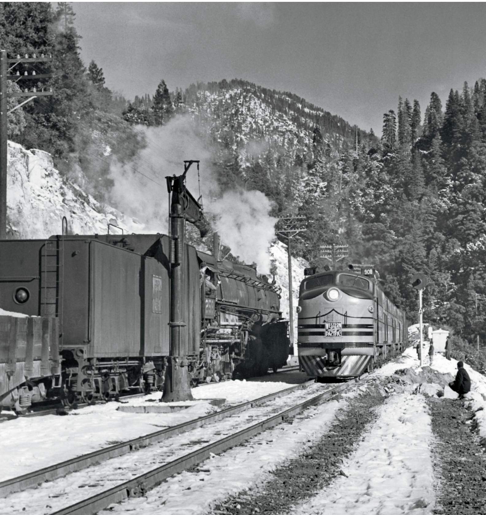
Western Pacific FT quartet 908, descending California's Feather River Canyon in early 1950, gets a wave from the engineer on 2-8-8-2 259 in a siding as other employees, at right, help with the "roll-by." Delivered in green and yellow, the FTs now wear "Zephyr orange" and black. WP was the second road to order FTs, after Santa Fe; its 111-unit F fleet totaled 48 FTs (12 A-B-B-A sets) plus 63 total F3s, F7s, and FP7s. Two F7s served into 1983.
